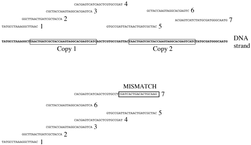
Fig. 8.14. Assembly of a DNA strand with repetitive structure. The true DNA strand contains two identical copies of sequences, marked by rectangular boxes, named copy 1 and copy 2. In the upper par of the figure this DNA strand is covered by seven reads, 1, 2, . . . , 7. The lower part shows the process of DNA assembly by a heuristic method of growing a contig from reads. Reads are added in the order 1, 2, . . . , 7. Note that reads 6 and 7 are positioned incorrectly, owing to the repetitive structure of the DNA strand, and that when read 7 is added a mismatch occurs
